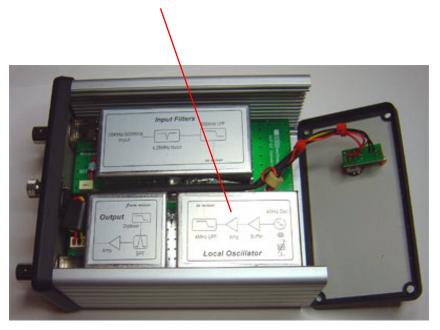
Switch ON the converter. Allow at least 30 minutes of warming time before adjusting at room temperature.
